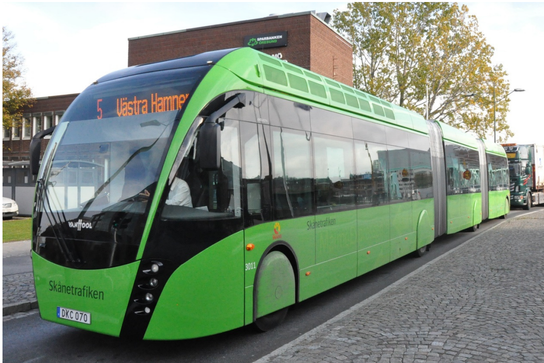
Figure 12: One of 15 gas/electricity hybrid “tram-buses” that are 24 meters long in the city of Malmö. This is one of 2,200 buses in Sweden running on a mixture of 58% biomethane and 42% natural gas. 2,200 buses correspond to 16% of all buses in Sweden.
