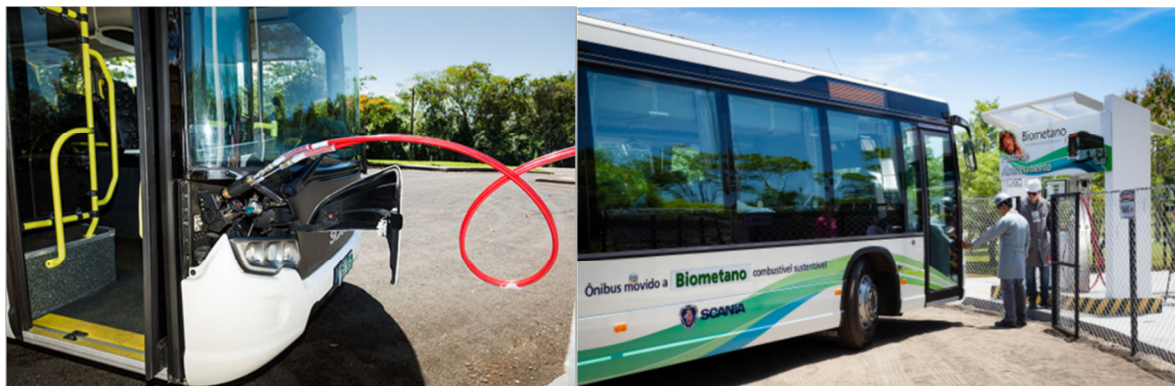
Figure 3: The first Scania Euro 6 bus operated with biomethane from food production in Brazil
